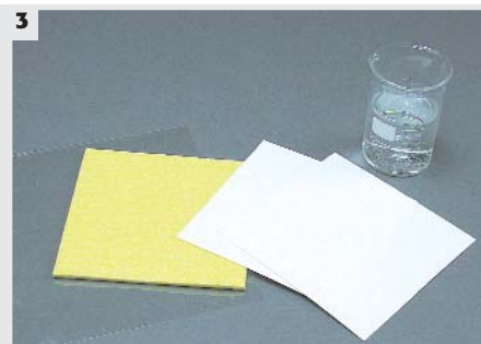
3 Moisten the sponge and the filter paper with 37 cl water.
