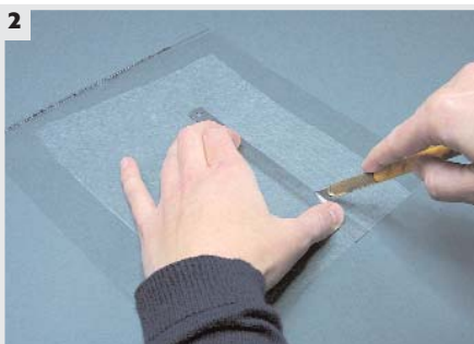
2 Score and cut the tissue with a knife into small strips. The width of the strip is your choice. Do not cut through the polyester film.
