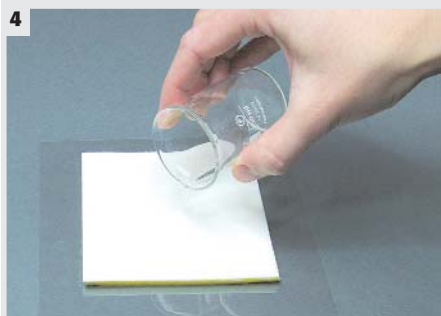
4 It takes about 10 minutes for the water to disperse evenly in the blotter system.
